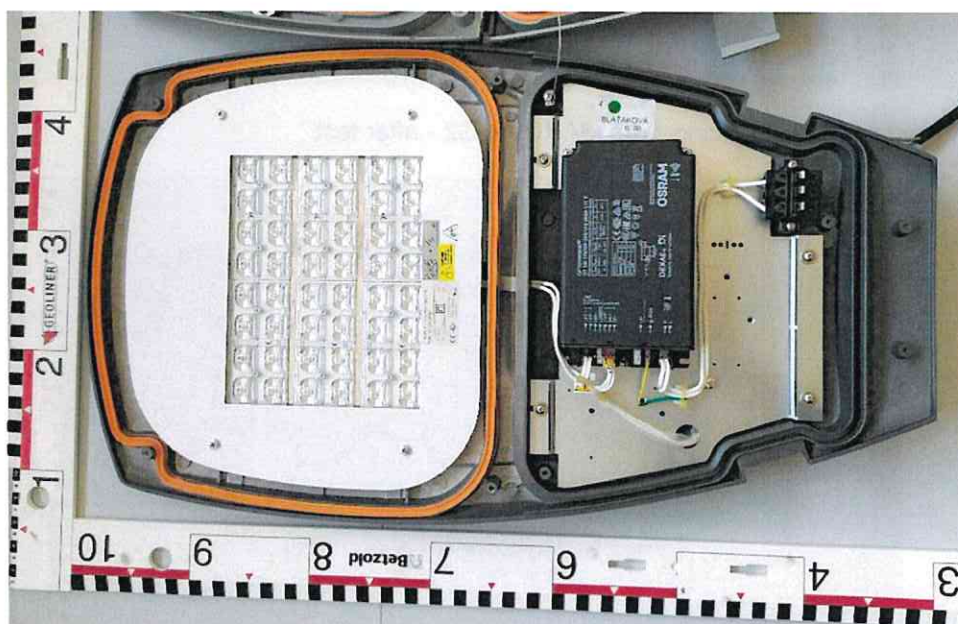
Open luminaire MARUT L G2 - after test
