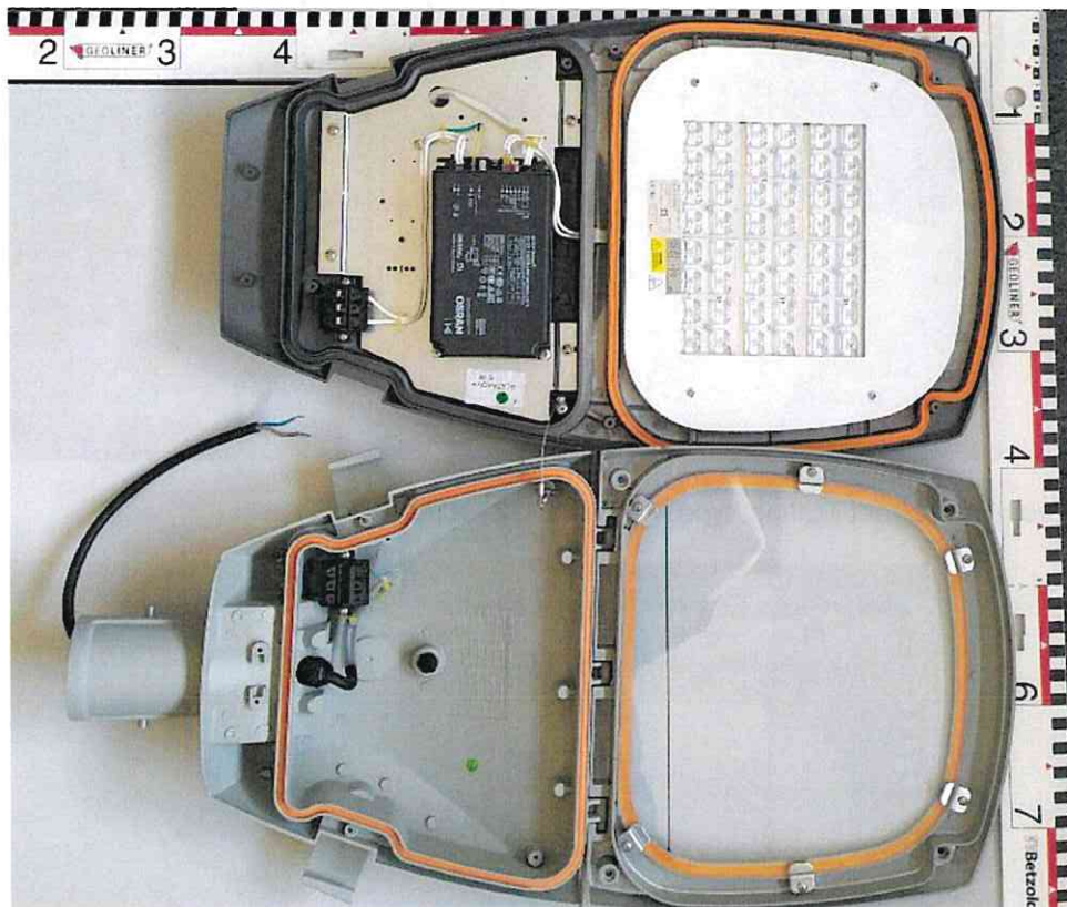
Open luminaire MARUT L G2 - after test
