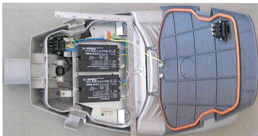
Open luminaire MARUT XL G2 - after test
