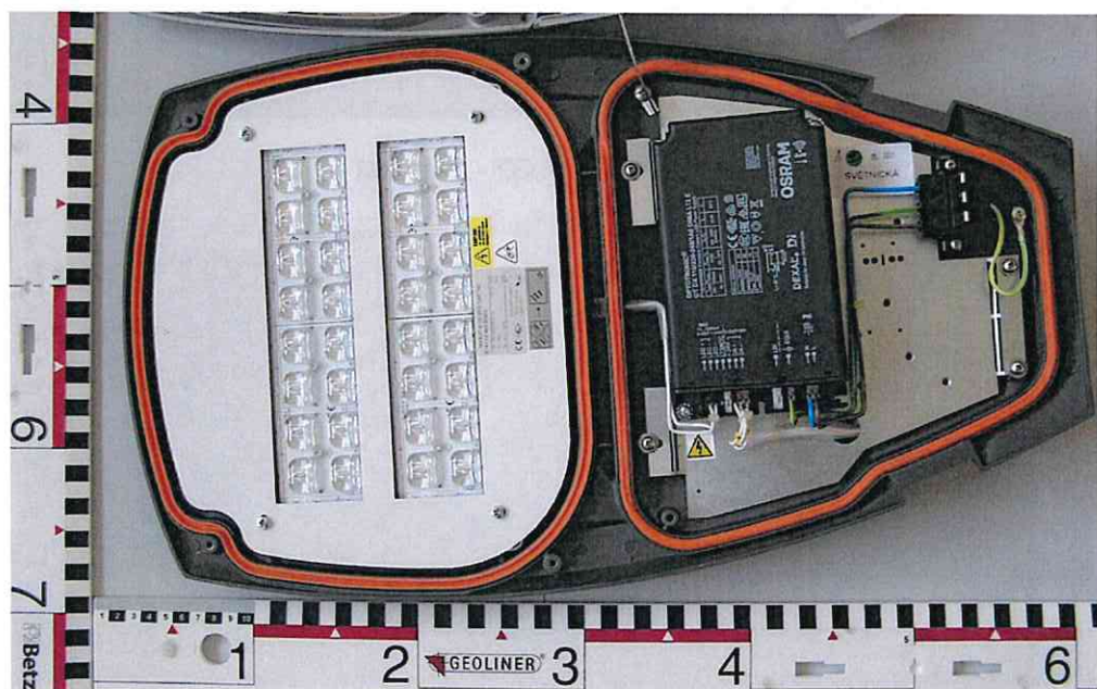
Open luminaire MARUT M G2 - after test
